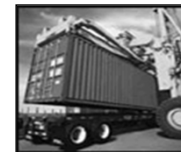
Mounting of container on a chassis.
